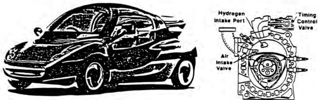
Figure 1. Japan's Mazda HRX Car and its Wankel engine.
